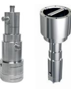
Designed to operate subsea at depths up to 3000m (10,000ft) these regulators can either use the external seawater pressure as a reference pressure or be completely sealed to operate at topside ambient pressure conditions, thus are completely unaffected by external pressure conditions. A version of the regulator is also available with a 'bucket handle' to allow subsea adjustment by ROVs
